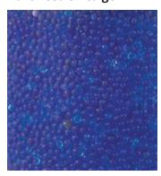
Desiccant removes water from air prior to it entering your system, tank or equipment.
